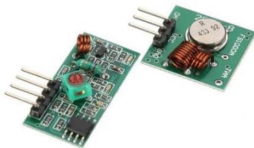
Gambar 2.6 Modul RF Rx/Tx 433 MHz
