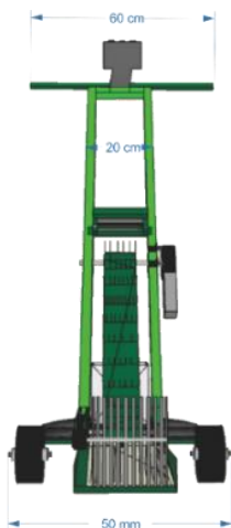
Figure 6. Front view of trolley design
