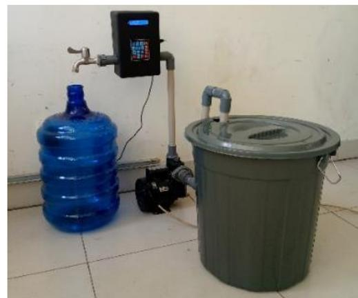
Gambar 5. Set Up Alat Monitoring Debit Air Pada Pengisian Air Galon Mineral
