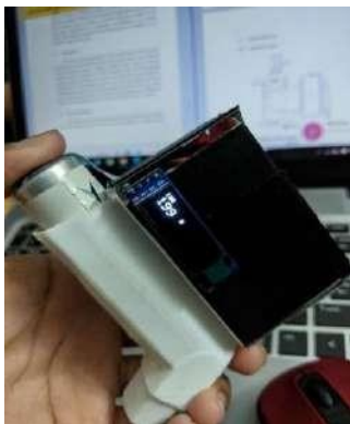
Figure 11: Dose Displayed At OLED Display When Pressure Applied >37N
