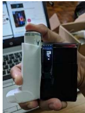
Figure 10. The Amount Of Remaining Dose And Percentage Of Battery Is Display In OLED.
