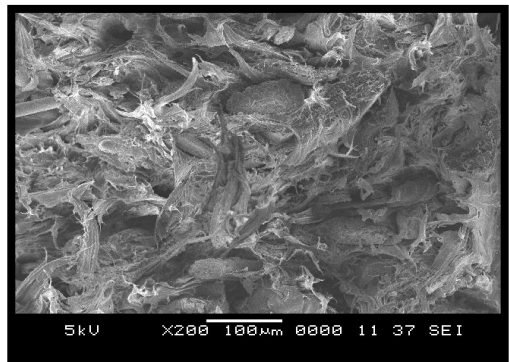
Figure 3: SEM micrograph at 200X magnification depicting the tensile fracture surface of Eco Bioplastics Packaging biocomposites compatibilized with MAPE
