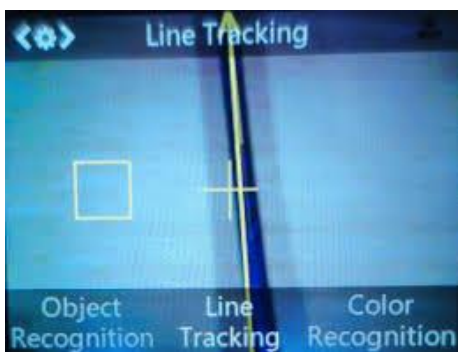
Figure 6. Line tracking with huskylens camera
